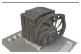
When dismantling the 135mm fan (2), push the notches of the fan clips (17) away from the fan.
