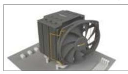
When dismantling the 135mm (2), push the notches of the fan clips (17) away from the fan.
