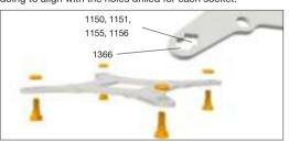
For fixing the backplate screws onto the Intel backplate use the O-rings (14). Once assembly of the Intel backplate for the respective Intel socket is complete, position it under the motherboard. Make sure that the backplate screws are precisely positioned inside the motherboard holes.
