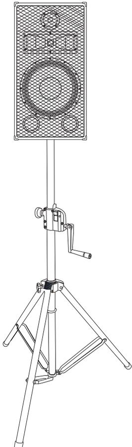
The speaker-system may only be installed on a stand or speaker stand if the original speaker-system is equipped with an appropriate flange.
