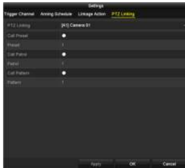
Figure 8-7 Set PTZ Linking of Alarm Input
