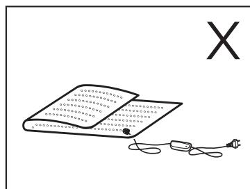
The electronic components inside the controller may cause the controller slightly warm when the heating pad is in use. Therefore, the controller must not be covered or placed on top of any heating sources when it is in operation.
