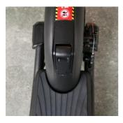
Use your hand to hold the arrow position and lift the foot pedal upward.
