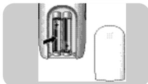
**2** Insert the two 1.2V AAA size NiMH rechargeable batteries (supplied), noting the + and – configuration inside the battery compartment.
