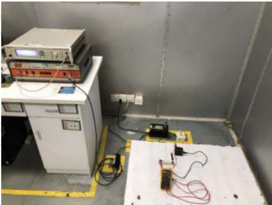
RADIO-FREQUENCY CONTINUOUS CONDUCTED IMMUNITY TEST SETUP
