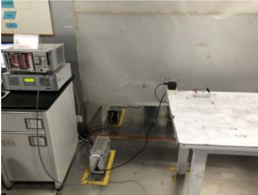
CONDUCTED DISTURBANCE TEST SETUP
