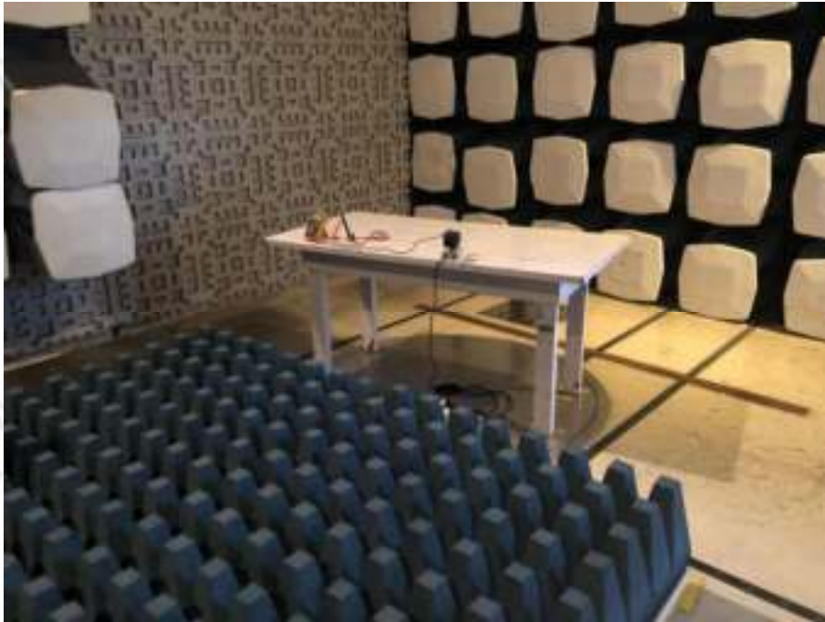
RADIO-FREQUENCY ELECTROMAGNETIC FIELD TEST SETUP
