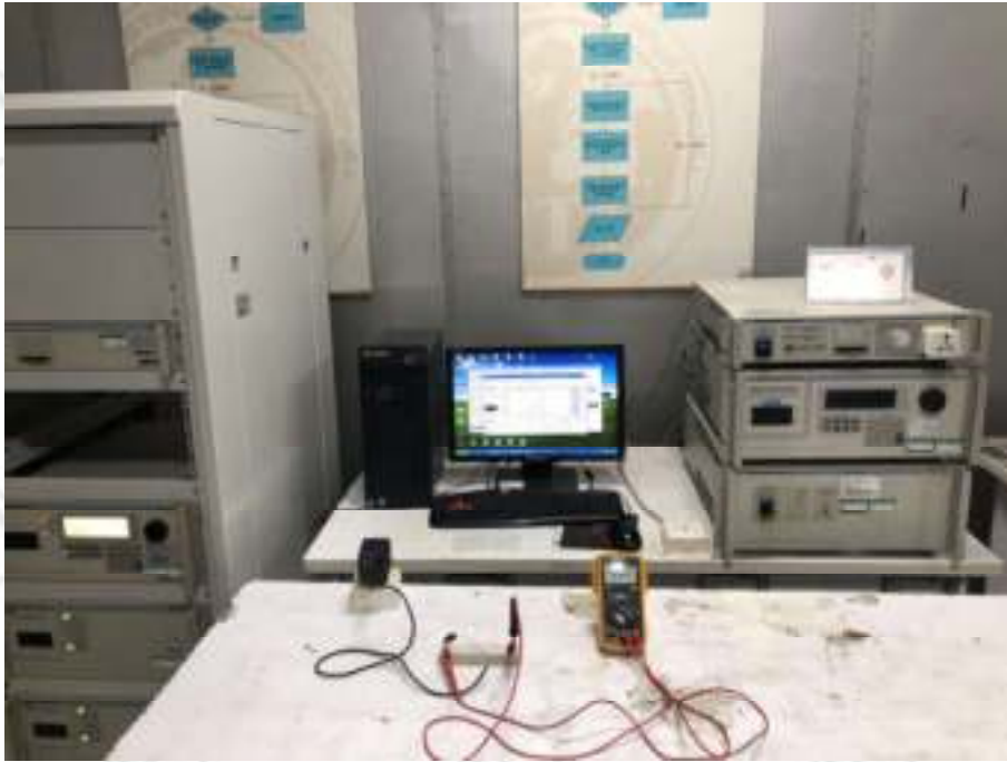
VOLTAGE DIPS AND INTERRUPTIONS TEST SETUP
