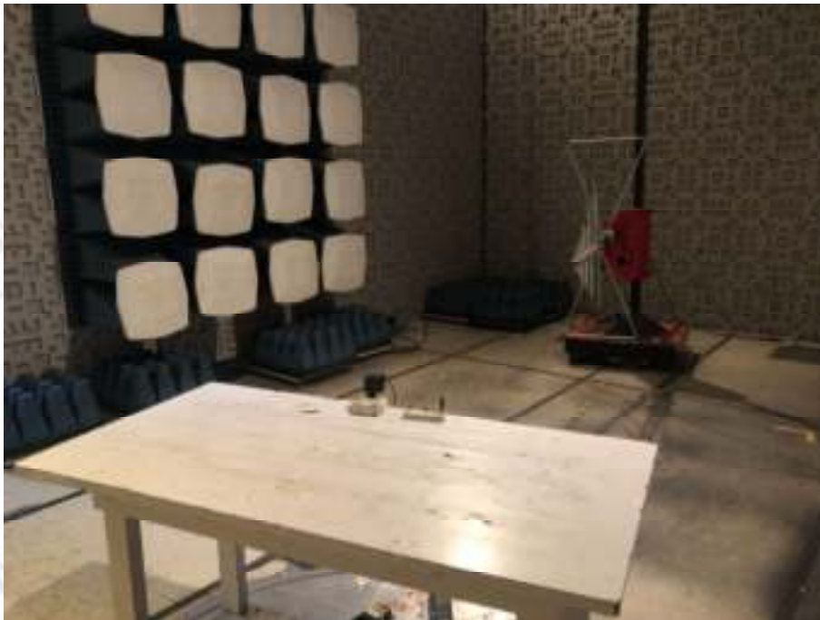
RADIATED DISTURBANCE TEST SETUP
