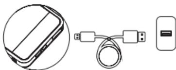
Connect the powerbank to power adapter USB port with the supplied USB to Micro-USB cable directly.
