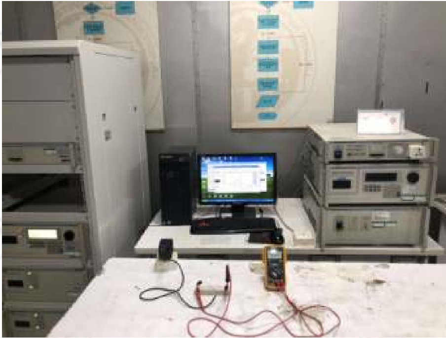
VOLTAGE DIPS AND INTERRUPTIONS TEST SETUP
