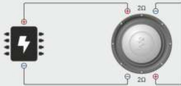
Serial wiring → 4 Ohms
