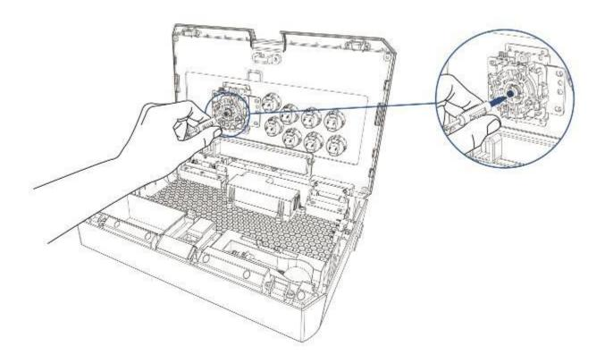
4. Rotate the Ball Top Joystick Grip until it is removed from the joystick shaft.
