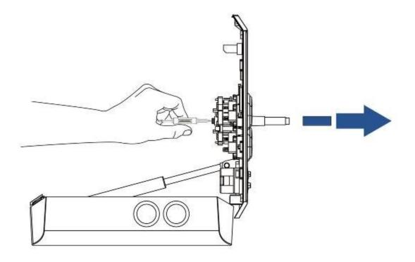
6. Rotate the Bat Top Joystick Grip onto the joystick shaft until it is securely fastened.
