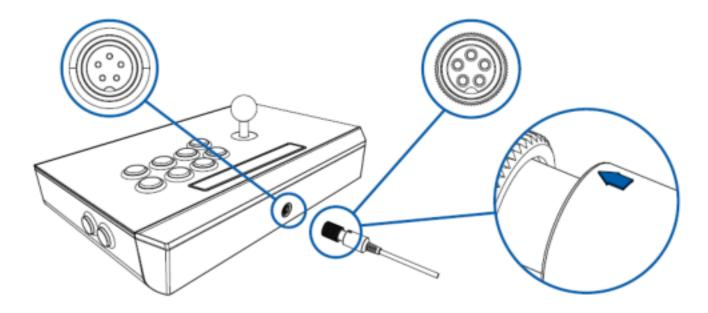
6. Rotate the screw collar clockwise until the detachable cable is firmly connected to the Razer Panthera.
