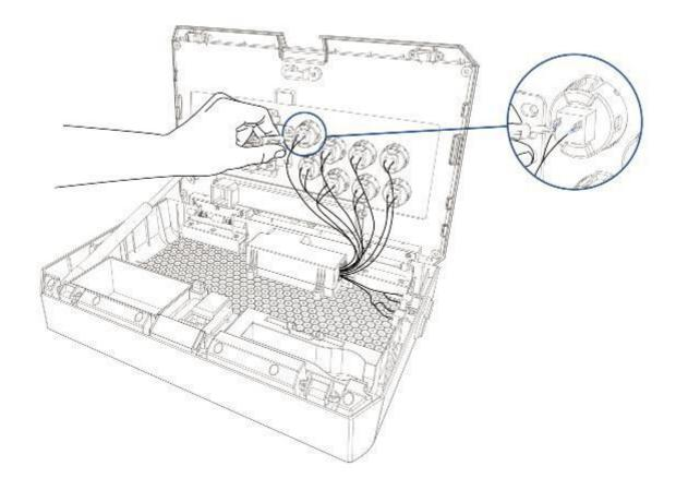
4. While holding the action button's fastener, push the action button out. You can use the screwdriver to push the fasteners in more easily, if needed.
