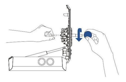
5. Remove the shaft cover from the joystick shaft.
