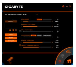
Users could also choose CUSTOMIZED for fan setting, and move the white dots on the line chart to adjust fan speed and temperature.
