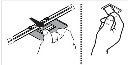
**4.2 NON-washable activated charcoal filter** - The saturation of the **charcoal filter** occurs after more or less prolonged use, depending on the type of cooking and the regularity of cleaning of the grease filter. In any case it is necessary to replace the cartridge at least every four months. The charcoal filter may NOT be washed or regenerated.
