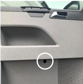
4. Remove the single T25 Torx screw located in the centre of the door card
