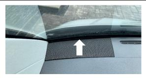
15.To remove the factory tweeter (if fitted) first use a trim removal tool to remove the dash cover. Lift the front edge first and remove completely
