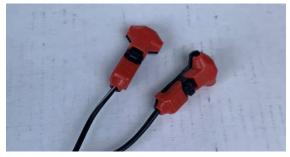
18. For vehicles that are not fitted with factory tweeters in the dash, the OPTI1C tweeter wires will need to be routed to behind the stereo. Connect the T Crimp connecters as shown to the Tweeter wires and clamp closed using pliers or similar.
