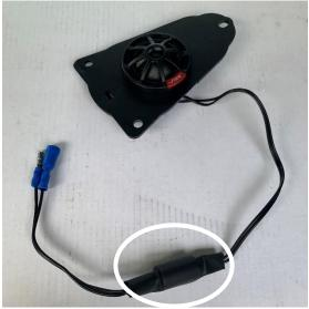
21. Cut back the tweeter wiring ensuring the crossover/capacitor remains in-line with the positive wire (Black/White).
