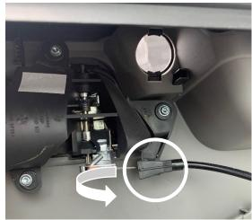
6. With the door card fully released from the door, unplug the window/door switches, and release the door opening cable. This is released by unclipping the front edge and sliding it back out of its locating channel. Once released, unhook the metal cable
