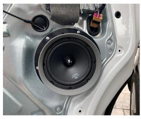
14. Connect the speaker spade terminals to the woofer ensuring the polarity is correct (Red Positive +, Black Negative -) Line up the holes and silicone baffle and use the screws provided to secure to the speaker adaptor
