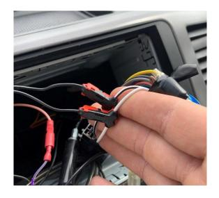
19. Connect the T-Crimp connectors to the stereo front speaker output wires. Take special care to ensure the polarity is correct so power correctly flows through the tweeter crossover. If unsure refer to your stereo user guide or wiring diagram. (Tweeter wiring, Black/White – Positive +, Black – Negative -)
