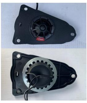
17.Before fitting the new tweeters, please make sure the crossover or capacitor is used to protect the tweeter. (See Section 21 for details.)
