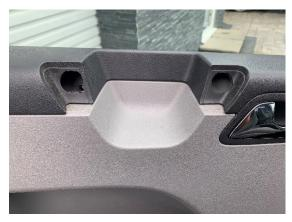
3. With the Torx screws removed, remove the handle completely from the door card.
