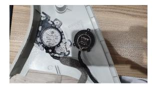
16B. Once removed the Tweeter is now able to be removed. These are plastic welded into place from factory and can easily be removed with the use of heat and a small amount of pressure.
