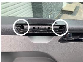
Using a trim removal tool, remove the plastic trim from the centre of the door handle then remove the two T25 Torx screws located behind. (We recommend using the VIBE CLTRT-V7 trim removal tools available from any VIBE authorised dealer)
