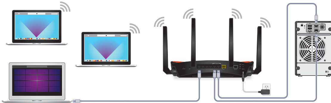
Figure 7. Ethernet port aggregation
