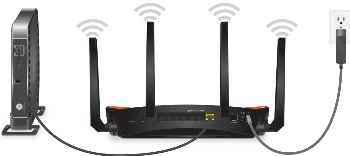
Figure 6. Cable your router
