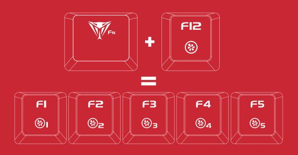
Press FN+F12 for F1-F5 to enter a blinking state in preparation to record a custom key configuration. Once in this blinking state, select any of the F1-F5 keys to assign a configuration.
