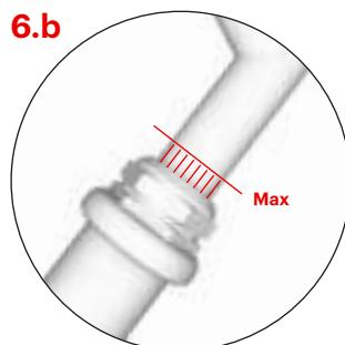
The highest possible height of the handlebars is marked with vertical grooves, at the maximum height the grooves should be visible only partly.
