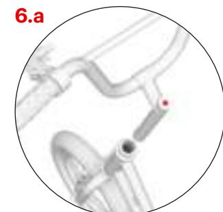
Insert the stem into the frame tube of the scooter and adjust the handlebar height taking care not to position it above the marked line, see pic. 6.b. Make sure that the handlebars are straight and then tighten the screw on the stem.
