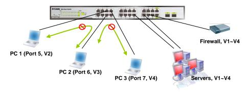
Figure 66 – Configuration > 802.1Q VLAN > Asymmetric VLAN Example
