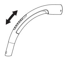
Suction power is also adjusted using the slide control on top of the vacuum cleaner. The symbol on the control indicates the direction for maximum and minimum suction power.
