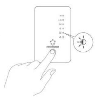
3. The devices will establish a connection. The extender's green WPS LED should display on for 30 seconds to indicate a successful connection.
