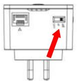
If you are using the extender in a small or medium sized space, you may not need the full power of the wireless radio. Try it, and determine if you still have sufficient Wi-Fi coverage using green mode. If so, you can save some energy.
