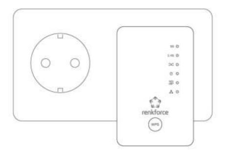
2. The green power LED will flash while the extender is starting up. The device is ready when the green power LED displays on.
