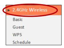
The "2.4GHz Wireless" & "5GHz Wireless" menu allows you to configure SSID and security settings for your Wi-Fi network along with a guest Wi-Fi network. WPS, access control (in access point mode) and scheduling functions can also be managed from here.
