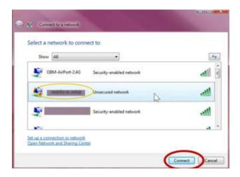
**3.** After correctly entering your password, you will be successfully connected to the EW-7476RPC's wireless network.
