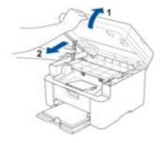
If you install a new genuine Brother toner cartridge but the **Replace Toner** message remains, the drum unit and toner cartridge assembly is not installed correctly. Take the drum unit and toner cartridge assembly out of the machine and put it back in.
