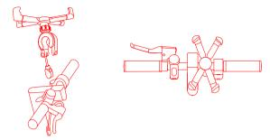
Rotate hand screw to the slot of buckle and tighten hand screw, adjust the phone holder to the appropriate angle, and tighten adjustment nut.
