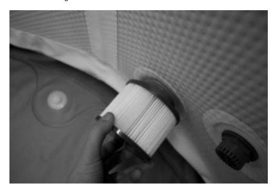
14. Add Filter Protector Cover onto Filter Cartridge.
