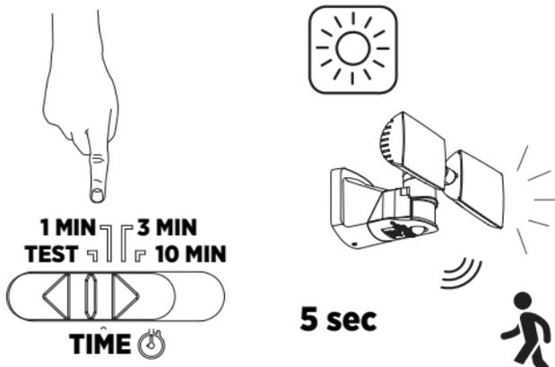
To adjust the detection zone in daylight. When the sensor detects movement the light turns on for 5 sec.
