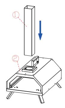
Insert the chimney in the direction of the arrow.
