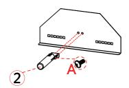
Use two M5x12(A) screws to fix the handle to the door.
