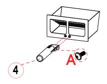
Use two M5x12(A) screws to fix the handle to the firebox.
