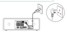
Connect the power cord to the wall socket.
