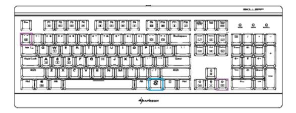
Any number of keys on the SKILLER MECH SGK3 can be illuminated without software. To do this, first press and hold the SKILLER key then press the SET key . The "Customize" lighting effect is now selected. Press the key combination again to enter the lighting programming. The LEDs above the number block will flash as an indicator.
