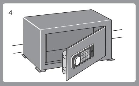
GB To check that your PIN code has been accepted operate the lock three times without closing the door. If unsure repeat the steps above.
