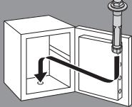
GB The safe must be anchored before being use.
