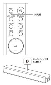
Press and hold the BLUETOOTH button on the Bar Speaker and INPUT on the remote control simultaneously for 5 seconds.
