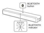
If pairing is not performed for 5 minutes after the system enters the pairing mode, the pairing mode is canceled. In this case, perform pairing from the start.
