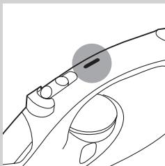
The safety auto-off function automatically switches off the iron if it has not been used for 30 seconds resting on its soleplate or 8 minutes resting on its backplate. The auto-off light will light up.
