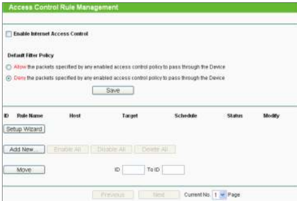
Figure 5-48 Access Control Rule Management
