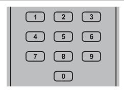
Using the direct-entry numeric keypad (0 to 9) causes the C 568 to jump directly to the beginning of a numbered track and commence play. Thus, to play Track 5, simply press "5". To play Track 20, press "2" and "0".
