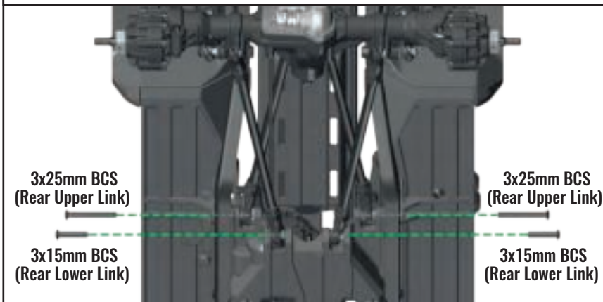
Install upper and lower suspension links to chassis
