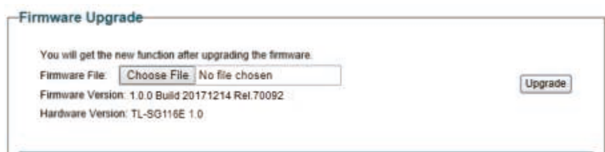
Figure 8-6 Being Ready to Upgrade the Firmware
