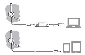
**IMPORTANT** Ensure that your 3.5 mm connector is fully connected to the headset controller.
