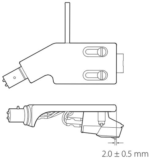
**4 Connect the shell lead terminals to the cartridge.**
