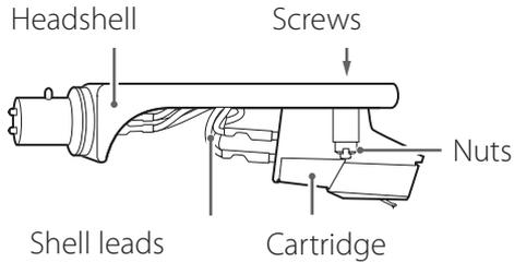
**1 Disconnect the shell lead terminals from the cartridge.**
