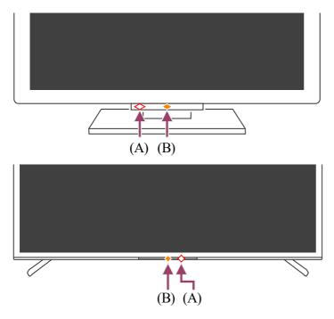
(A) Voice function LED (On the left side or center right at the bottom of the TV. Only TVs with a built-in MIC.\*)
