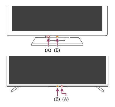
(A) The voice function LED is located at the bottom just left of center or center right of the TV.(B) The LED located at the bottom center of the TV lights up amber when hands-free operation is available.
