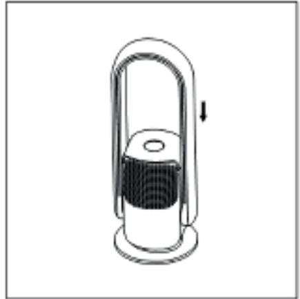
Reinstall Top Cover, the magnetic-lid will snap into place automatically.
