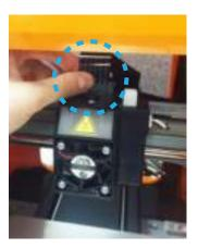
2 Insert the black ribbon connector to complete the installation.
