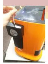
1 Ensure that the guide tube has been tightly inserted into the port.
