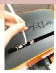
2 Feed the guide tube through the slot at the top of the printer to the extruder module.
