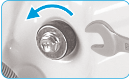
Loosen the 4 transport bolts with a spanner.
