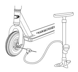
Using a bicycle-style tire pump equiped for a Schrader-type valve, inflate the front tire to the correct PSI indicated on the sidewall of the tire.
