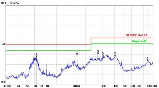
Site LAB Limit: EN 55032 CLASS B Polarization: Horizontal Temperature:
