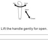
Turn lever around to adjust water temperature.
