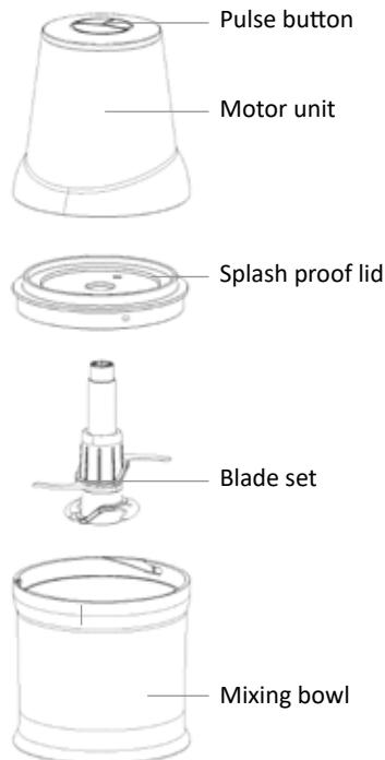
The blade set consists of two parts. A base part with two blades and an extra part also with two blades. You can slide the extra part over the shaft and click it onto the base part. In this way you will have 4 blades for extra fine chopping. See figure.
