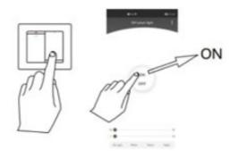
Step 2, turn on the light, press the ON in the APP immediately, then the pairing starts
