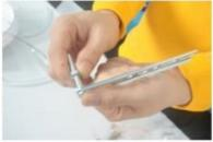
7, assemble flat-headed screws to the hanger with nuts in, but don't lock up yet
