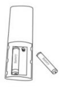
Step 1, put batteries in the remote
