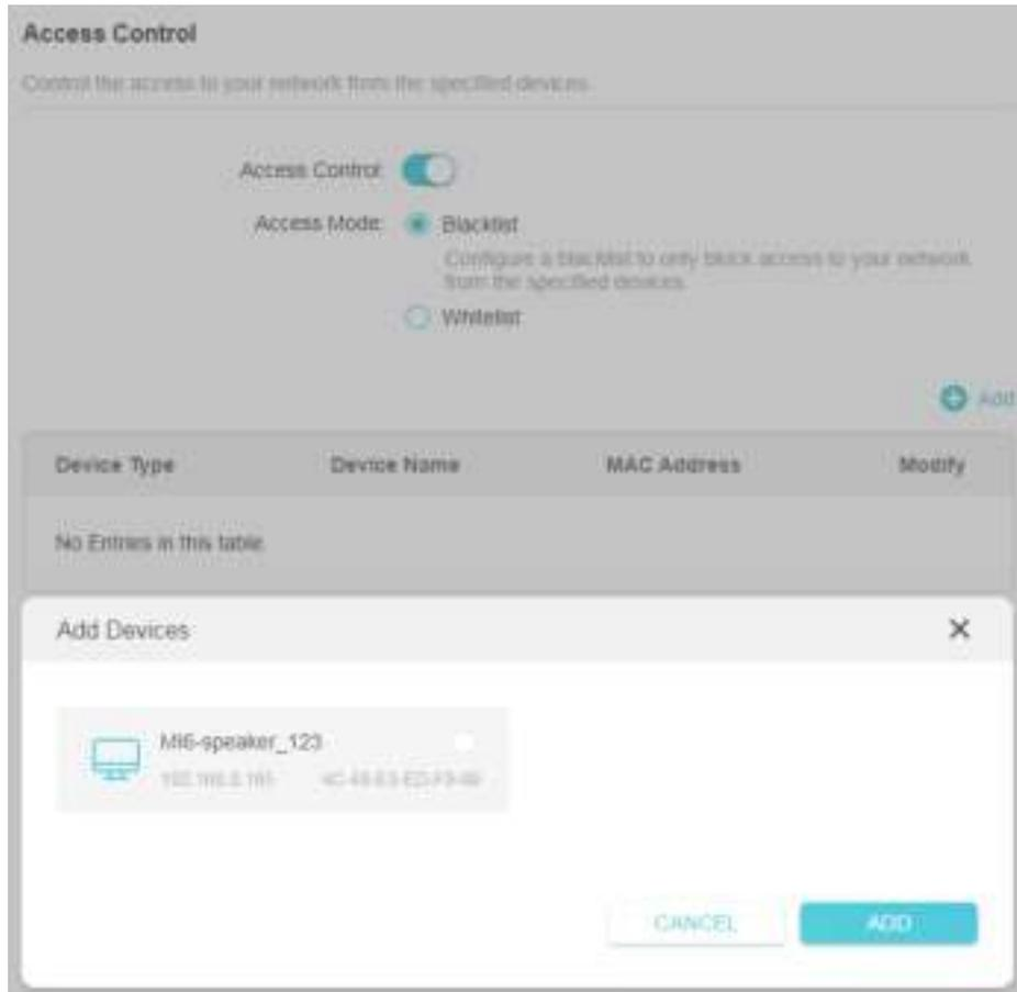
2. Select the device to be blocked in the [Add Devices](#) table.
