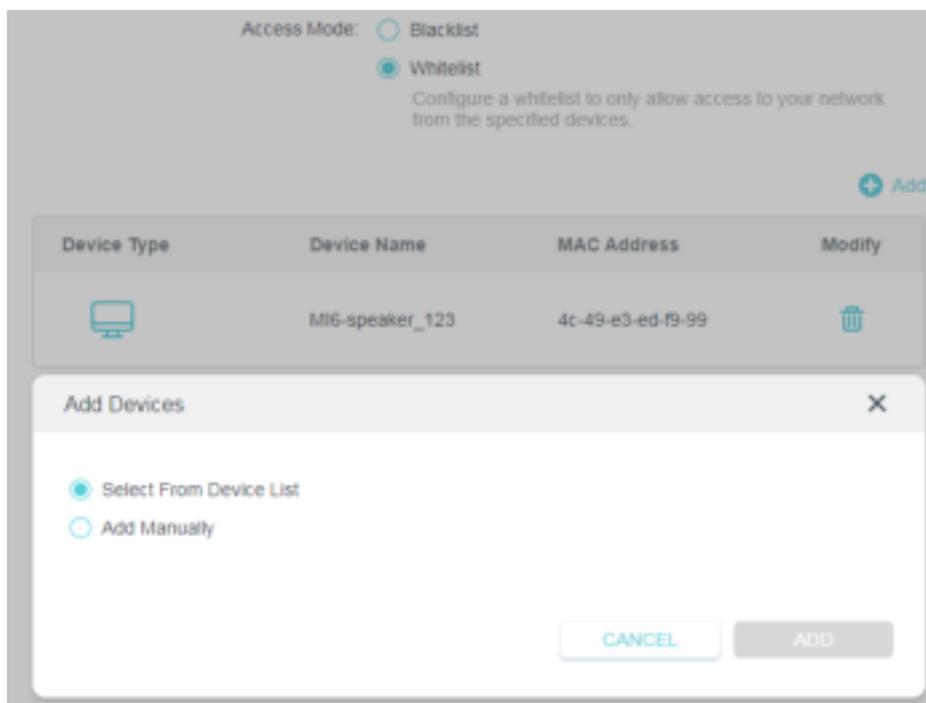
2. Select from the Device List or add devices manually in the [Add Devices](#) table. Enter the [Device Name](#) and [MAC Address](#) if you add devices manually.
