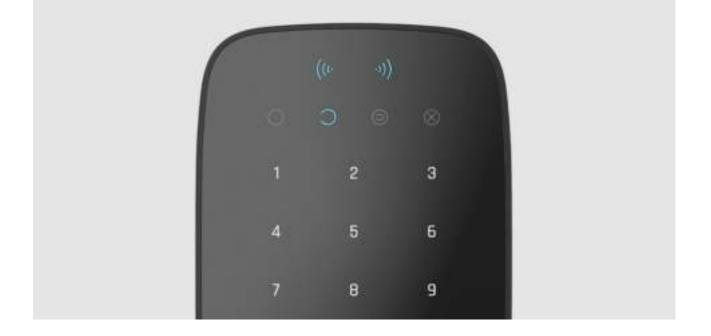
You can use the KeyPad Plus without ambient lighting as the keypad has a backlight. The pressing of the buttons is accompanied by a sound signal. The backlight brightness and keypad volume are adjustable in the settings. If you do not touch the keypad for 4 seconds, KeyPad Plus reduces the backlight brightness, and 8 seconds later goes into power-saving mode and turns off the display.
