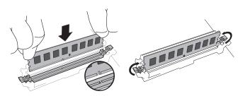
Using firm, even pressure, push DIMM into slot until clips snap into place. Do not assist clips.
