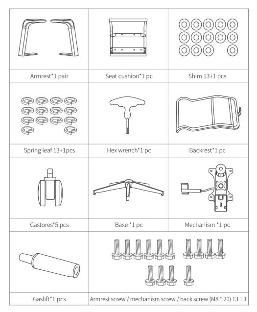
Note: before installing the chair, please sort the screws and measure the screw length for installation.
