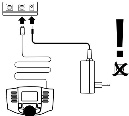
Once the Mobile Station and the switched mode power pack is connected to the digital connector box, the switched mode power pack can be plugged into a household current wall outlet.
