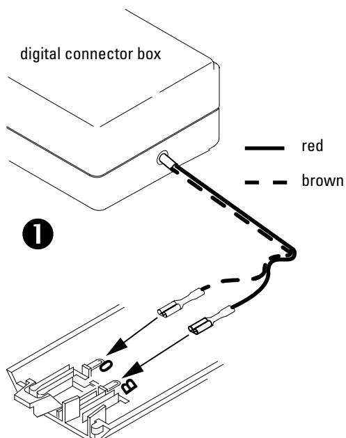
After the digital connector box is connected to a section of track, the track can be put together as shown in the following diagram.
